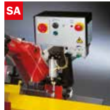
Discesa controllata Gravity down feed
